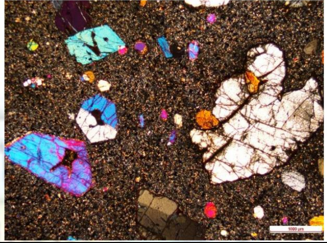
Photomicrograph 2: showing Large phenocrysts of olivine and clinopyroxene in very fine basaltic matrix showing porphyritic texture; under cross polarized light; 2X
