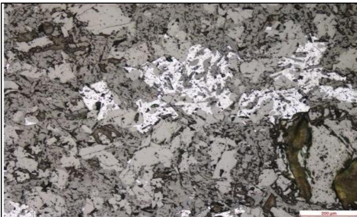
Photomicrograph 71: showing Anhedral magnetite intergrown with silicates; under reflected light and at 10X magnification
