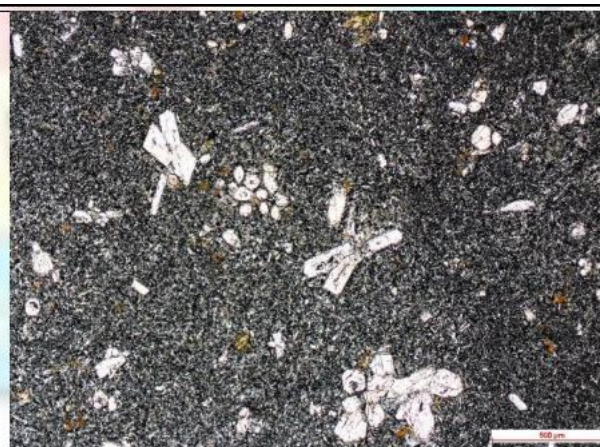
Photomicrograph 84: showing Clusters of phenocrysts within microlite and glass enriched matrix
