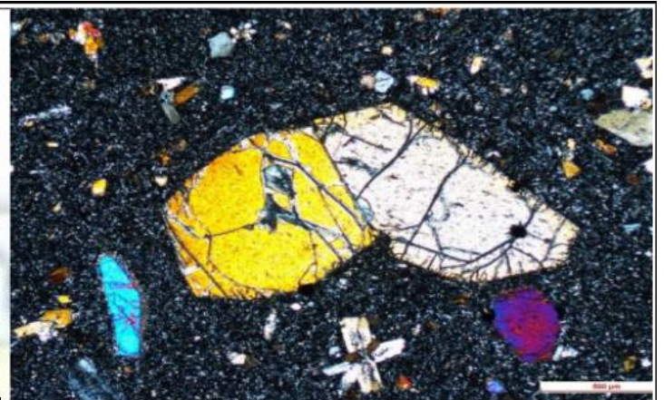
Photomicrograph 74: Large euhedral and fractured olivine phenocrysts; note the bimodal phenocrysts size distribution; magnetite rich matrix and phenocrysts of clinopyroxene forming star shaped cluster under cross polarised light
