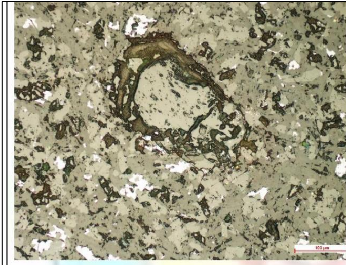
Photomicrograph 9: showing Small anhedral magnetites disseminated in matrix; under reflected light and 20X
