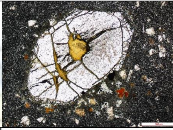
Photomicrograph 80: showing Olivine phenocryst altered along fractures by biotite; biotite also alters the matrix phases.
